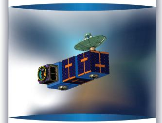
Orbital Replacement Unit based on Building Blocks for On Orbit Advanced Assembly of Space **Systems**
