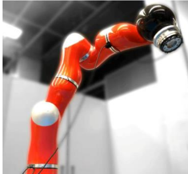
Fig. 10. Light-Weight -Robot with a force-torque sensor at the end effector (DLR)
